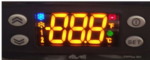
Fig. 4 . Indication and control elements of the controller Eliwell .
