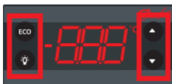
Fig. 10.1. Control elements of the Danfoss controller ERC 112 C
