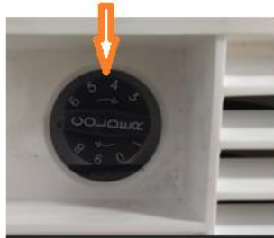
Fig. 3.1.1. The location of the thermostat in the side ventilation grille.
