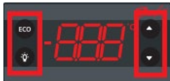
Fig. 3.1.2: Control elements of the Danfoss controller ERC 112 C.
